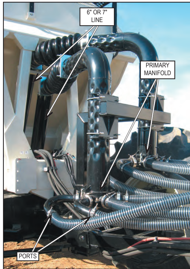
Figure 1 - Primary Line, Manifold and Ports (Double shoot is shown)
