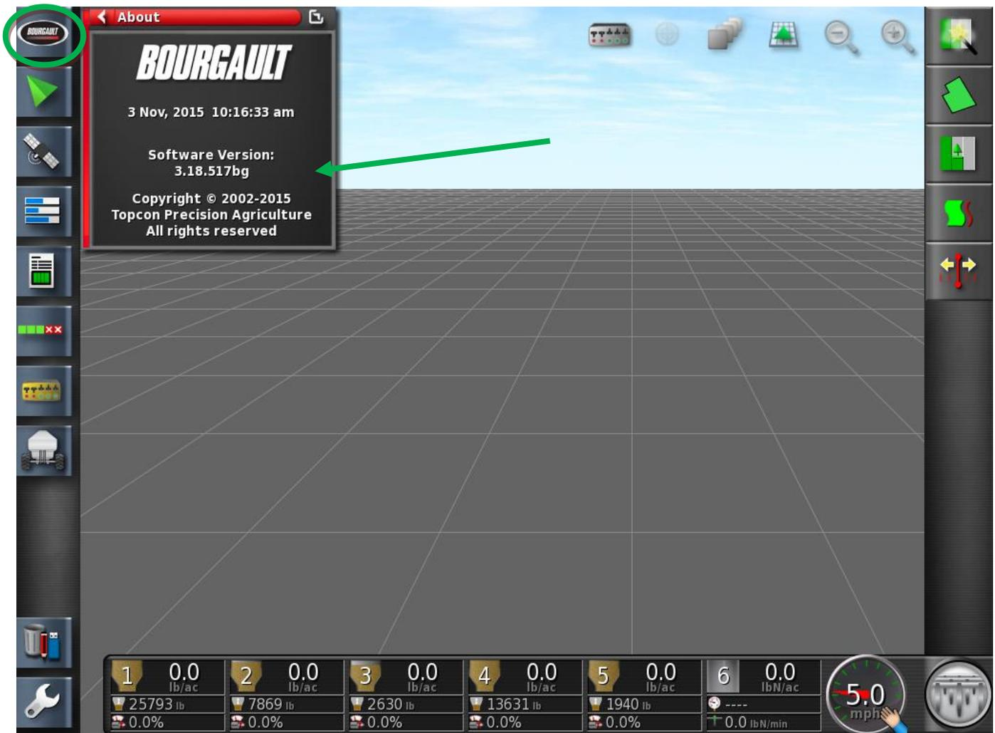
11. On main screen, click the Bourgault button in the top left hand corner. Ensure that the software version shown there is **3.18.517bg**
