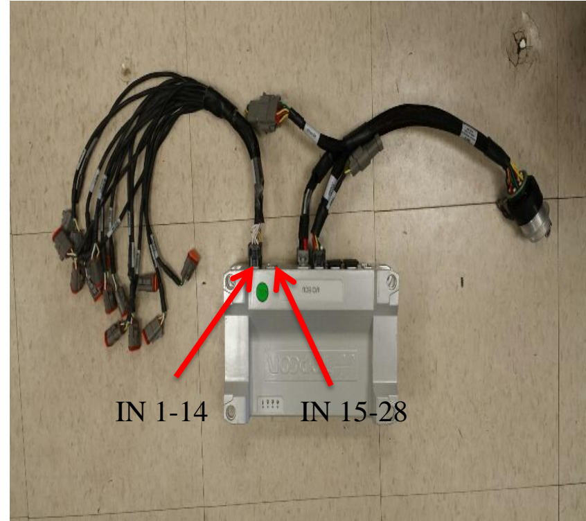
Plugs into the I/O on (IN 1-14) and if you have more than 16 sensors you will need another harness that will plug in on (IN 15-28)
